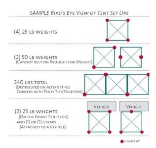
If a vehicle is used to secure one side of the tent, this can only account for half of the necessary weight, meaning for a 10 ft tent, you need an additional 50 lbs. on the front of the tent. You may not rely on product for weight.
